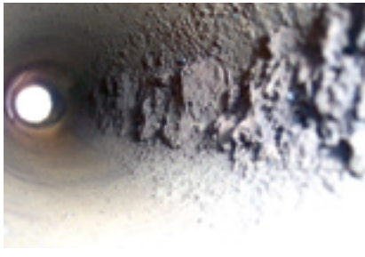
1. Test sample spool (left) is particularly important to monitor progress in chemical cleaning to rid deposits like that at the right (access presentation 2)
